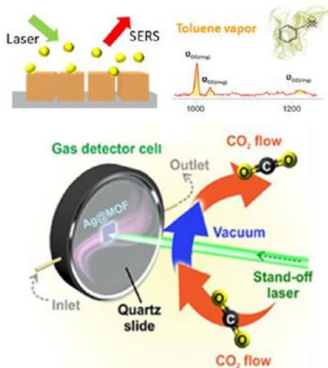
Figure 1. Scheme of our proposed SERS sensing system for hazardous gas/VOCs detection in designated plants.
